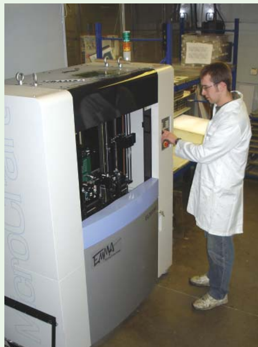
Above: the Microcraft EMMA moving probe tester improves high-layer count yields.
