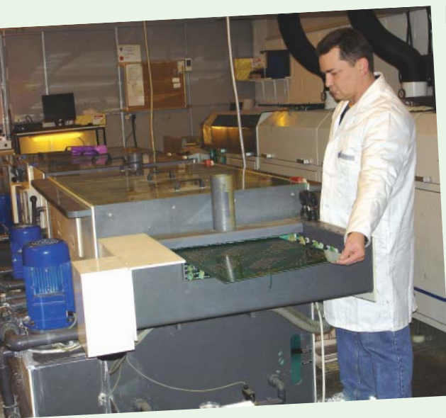
New solder resist developer line in action.
