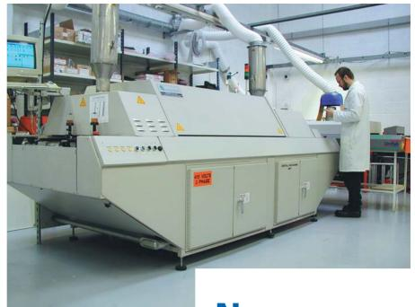
Consistent and repeatable processing is achieved using the newly installed Forced Air Convection Reflow Oven.
