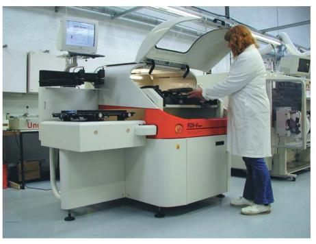
Vision alignment control on this newly installed machine enables very accurate solder paste printing and increases product reliability.
