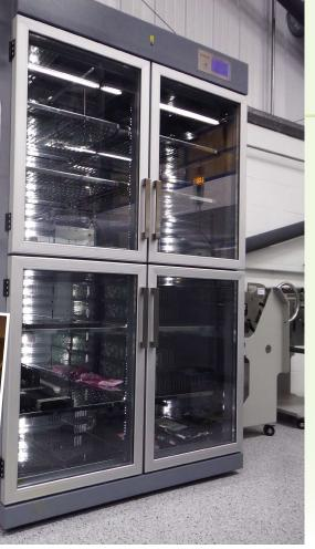
The new dry storage cabinet tightly controls humidity to under 2%.
